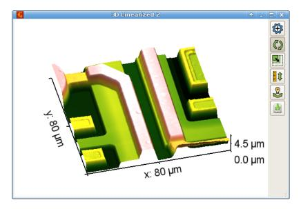
Three-dimensional OpenGL data display window with basic controls.
