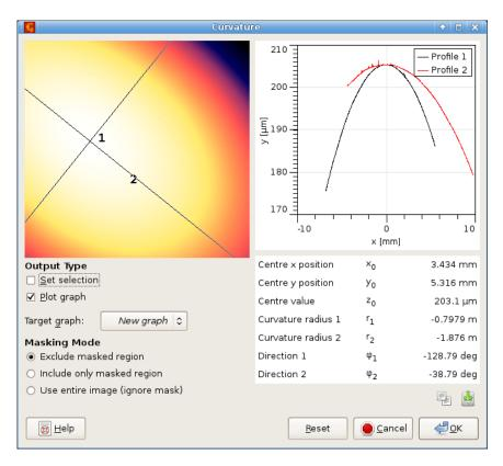
Curvature dialogue screenshot showing the strong deflection of a glass plate with a thin film with compressive internal stress.
