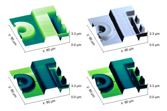
Visualisation modes of the 3D view. Top row: simple gradient and lighting. Bottom row: overlays with a different channel used for colouring (left without lighting, right with lighting).
