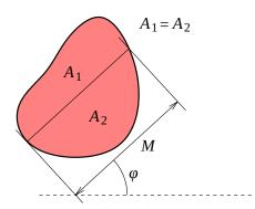
Determination of Martin's diameter at given angle.
