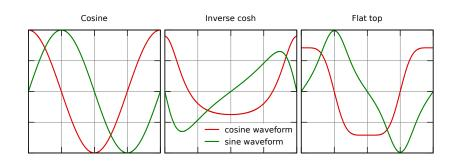
Sine and cosine wave forms for the available wave types. Only the cosine form is used for displacement images; the entire complex wave is used for intensity and phase images.
