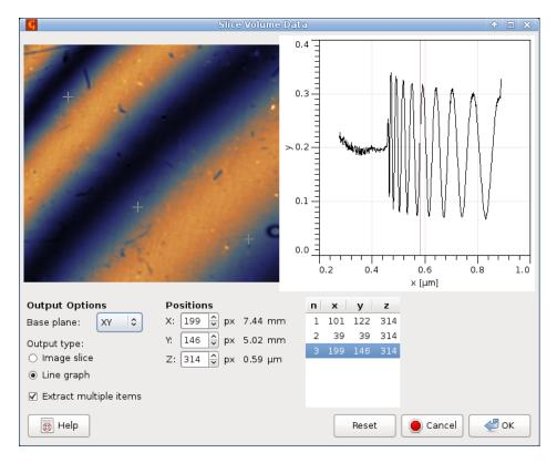
Screenshot of the Cut and Slice volume data processing module, showing the simultaneous extraction of three line profiles along the *z*-axis.
