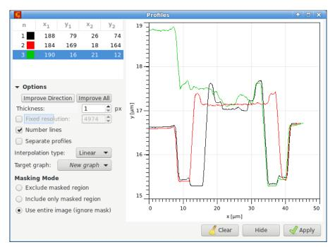
Profile tool with three extracted profiles and expanded options.
