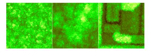
Artificial surfaces created by ballistic deposition: initial stage with relatively small correlation length (left); after correlations reached image size (centre); deposition starting from a microchip surface (right).
