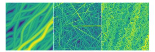
Artificial fibre surfaces: moderately deformed fibres, all oriented more or less in the same direction (left); many layers of thin straight randomly oriented fibres (centre); parallel fibres with high lateral deformation density (right).
