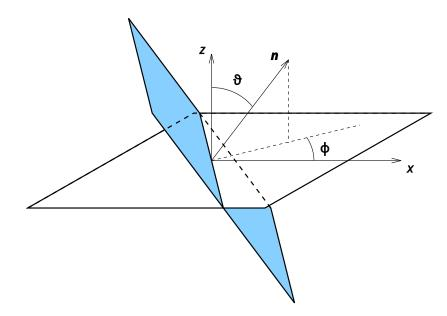
Surface facet (displayed blue) orientation measured as the anticlockwise angle from x-axis to the projection of facet normal vector **n** to xy plane.
