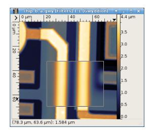
Screenshot of filter tool with median filter applied to a rectangular selection
