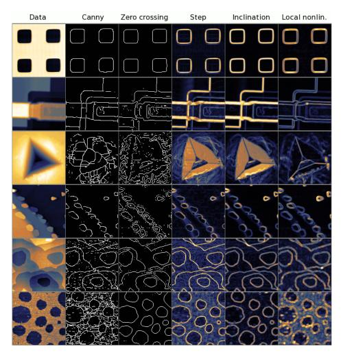
Comparison of step and edge detection methods on several interesting, or typical example data. Canny and Zero crossing are step detectors that produce one pixel wide edge lines, Step and Inclination are step detectors with continuous output, Local nonlinearity is an edge detector – the edge detection can be easily observed on the second and third row. Note zero crossing is tunable, it parameters were chosen to produce reasonable output in each example.
