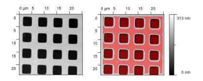
Certainty map obtained from standard grating. Note that the modelled tip parameters were taken from datasheet here for illustration purposes. (left) – sample, (right) – sample with marked certainty map.
