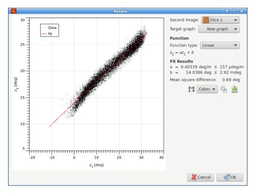
An almost-linear relation between two slices of volume MFM data at different heights, as displayed and fitted by the relation module.
