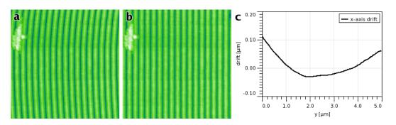
Drift correction example: (a) original data exhibiting strong drift in the fast scan axis, (b) corrected data, (c) calculated drift graph.
