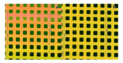
Path Level example: (a) uncorrected data with steps that the automated method may fail to correct, two suitable levelling lines are selected; (b) the result of Path Level application with line width 5.
