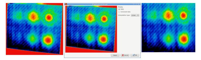
Perspective correction example. Left: original image exhibiting an perspective distortion. Centre: correction dialogue with the rectangle selected in the image. Right: corrected image.
