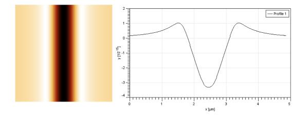
Stray field distribution above two parallel current lines with opposite current direction.
