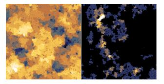
Wetting front images: a typical result with moderate coverage (left); initial stage of propagation (right).
