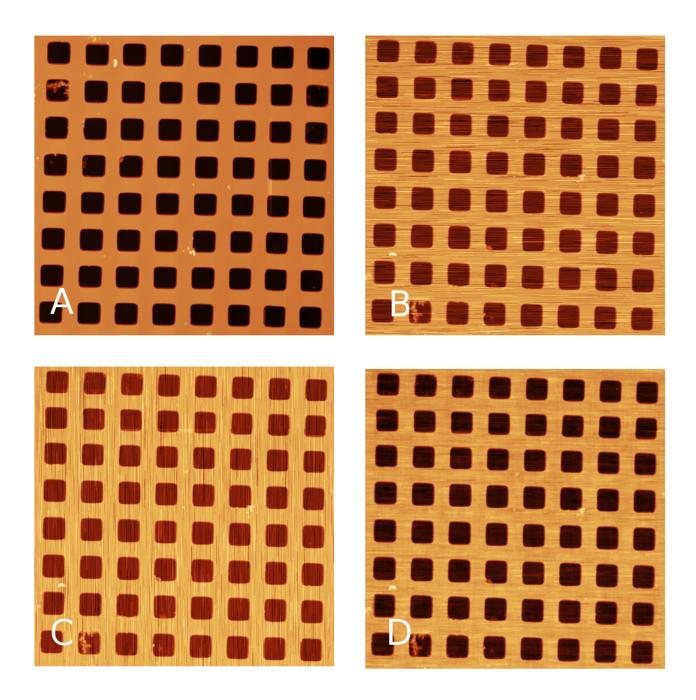
XY denoise procedure simulation: A) original data, B) simulated measurement in x axis, C) simulated measurement in y axis, D) denoised image.
