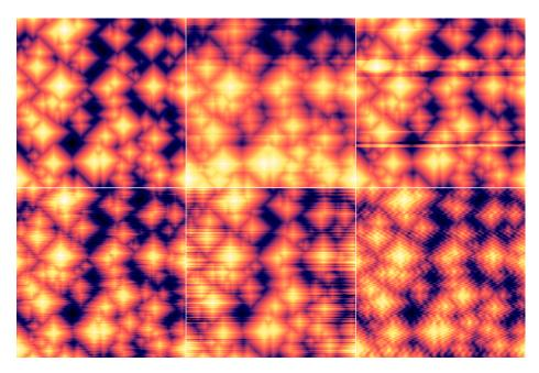
Different types of line noise added to an artificial pyramidal surface. Top row: unmodified surface (left); relatively sparse cumulative steps (centre); relatively sparse ridges (right). Bottom row: scars of mean length of 16 px and high coverage (left); tilt with small offset dispersion (centre); hum with default settings (right).
