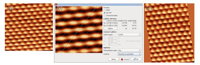
Affine correction example: (a) original image exhibiting an affine distortion, (b) correction dialogue with the lattice selected on the two-dimensional autocorrelation, (c) corrected image.
