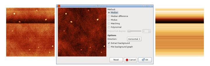
Line correction example: an image with defects (left), the row alignment dialogue previewing the median correction (centre), and extracted row background (right). Note the false colour scales are not the same in the three images.
