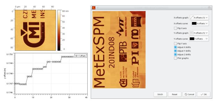
Volume data stitching example, showing one of 32 images taken on MetExSPM project test sample (manufactured by PTB), coarse movement stage data in X axis and the stitched data preview in the module GUI.
