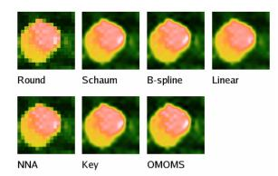
Illustration of the available interpolation types (the original pixels are obvious on the result of Round interpolation). All images have identical false colour map ranges.
