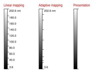
Rendering of the false colour map scale depending on the mapping type. For the standard linear mapping, whether full or fixed range, ticks with values are drawn. For an adaptive mapping the colour gradient is drawn the same, but tick positions correspond to the adaptive mapping and interior ticks are drawn without labels (to avoid overlapping labels). If a presentation is shown, the values are considered arbitrarily scaled thus no values and interior ticks are displayed.
