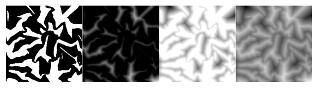
Euclidean distance transform example: the source mask shown as white on black, interior distance transform, exterior transform (with inverted greyscale for comparison) and the signed transform.
