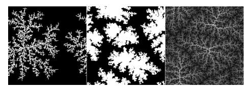
Artificial diffusion surfaces: sparse clusters with high sticking probability (left); dense clusters with low sticking probability (centre); multilayer fractal structures with high Schwoebel barrier (right).
