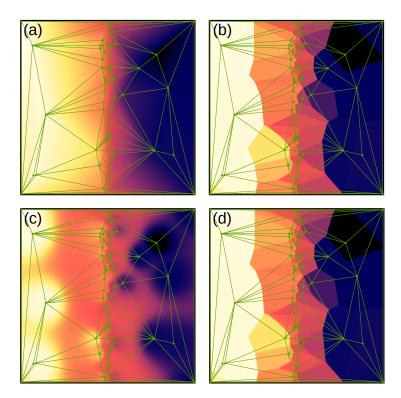
Delaunay triangulation displayed on top of (a) Linear, (b) Round, (c) Field and (d) Average interpolations of an irregular set of points. Since the points are sparse, Average interpolation is quite similar to Round, only a bit blurred.
