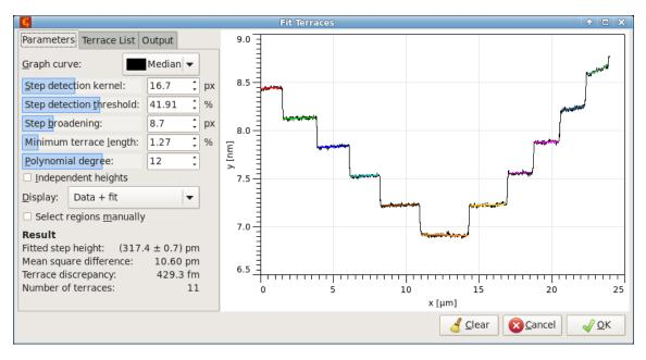
Terrace measurement from a profile, showing marked terraces for an amphitheatre structure formed by atomic steps on silicon.
