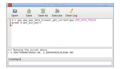
The pygwy console showing a simple script (printing the range of values of the current image) and its output.
