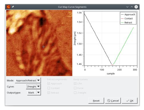
Screenshot of Cut to Segments module, showing typical segmentation settings for force-distance data.
