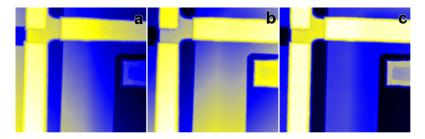
Facet Level example: (a) uncorrected, sloping data; (b) data levelled by standard plane fitting (Plane Level); (c) data levelled by Facet Level.
