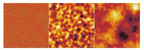
Artificial surfaces generated by spectral synthesis: a narrow range of spatial frequencies (left), Gaussian random surface (centre) and a fractal surface generated with power multiplier and *p* equal to 1.5 (right).
