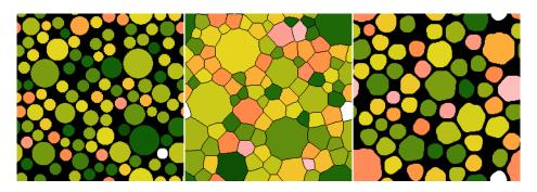
Artificial disc images: round discs with some height distribution (left); transformation to tiles (centre); erosion by opening filter (right).
