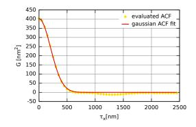
Autocorrelation function obtained for simulated Gaussian randomly rough surface (i.e. with a Gaussian autocorrelation function) with  $\sigma \approx 20$  nm and  $T \approx 300$  nm.
