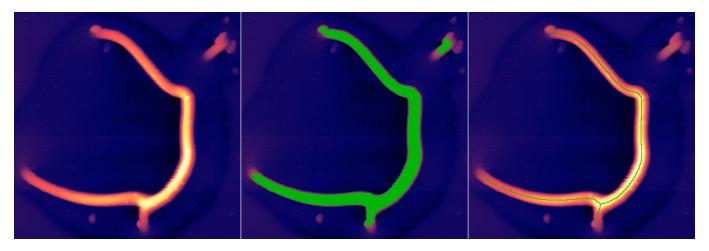
Mask thinning example: topographical image of buckling of a polymer film (left); the same image with a mask covering the bump on the surface (centre); and the same mask after thinning (right).
