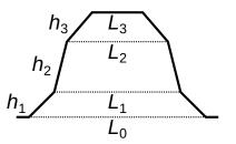
Widths and heights of the trapezoids forming the 3-level grating profile. Note that the widths are derived quantities, not direct fitting parameters.
