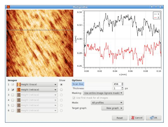
Basic usage of multiprofile module, with trace and retrace images selected as 1 and 2 and a the corresponding pair of profiles displayed in the graph.
