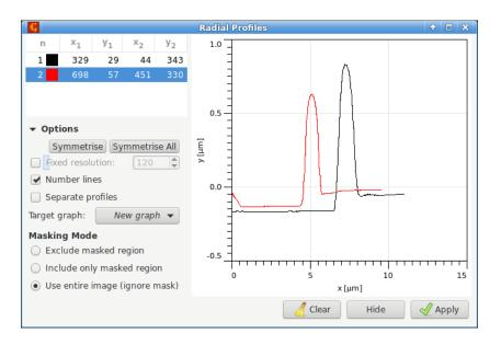
Radial profiles tool with two extracted selected profiles and expanded options.
