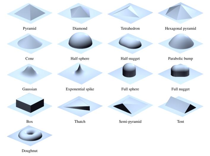
Parameters and options in the Shape tab control the shape of individual features:
