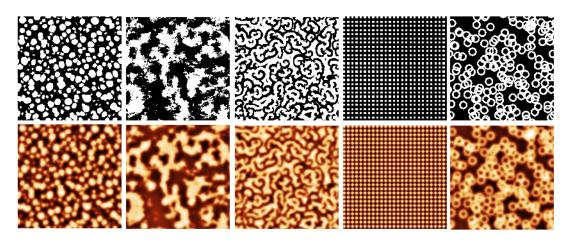
Result of data synthetic modules used for MFM perpendicular media simulation: columnar film, fractal roughness, Ising model domains, grating, doughnuts.
