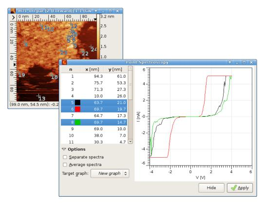
A data window with measurement points displayed and the point spectroscopy tool showing curves from three selected points.
