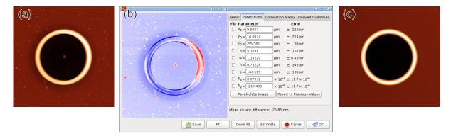
Shape fitting example: (a) original topographial data of a ring structure on the surface of a thin film, (b) fitting dialog with parameters on the right side and difference between data and fit displayed in the left part, (c) resulting fitted shape.
