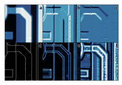
Presentation examples: (a) original data, (b) shading, (c) vertical Prewitt gradient, (d) Canny edge detection, (e) local nonlinearity edge detection, (f) local contrast improvement.
