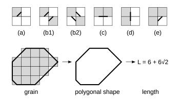
Contributions of pixel configurations to the estimated boundary length (top). Grey squares represent pixels inside the grain, white squares represent outside pixels. The estimated contribution of each configuration is: (a) h/2, (b1), (b2) h, (c)  $h_y$ , (d)  $h_x$ , (e) h/2. Cases (b1) and (b2) differ only in the visualization of the polygonal shape segments, the estimated boundary lengths are identical. The bottom part of the figure illustrates how the segments join to form the polygon.
