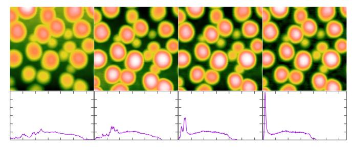
Flatten Base example: original image, levelled using Facet Level, levelled using Plane Level, levelled using Flatten Base. The original image is shown in linear colour scale, the levelled images are shown in adaptive colour scale. The graph below each image shows the corresponding height distribution (with the same axis ranges).
