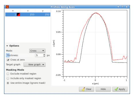
Profiles along axes tool with horizontal and vertical profiles crossing at zero and expanded options.
