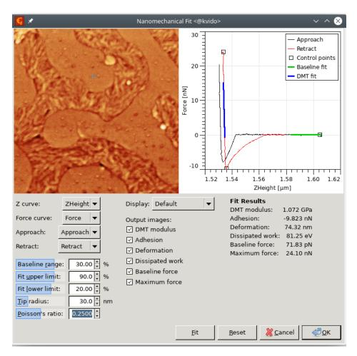
Screenshot of the Nanomechanical Fit module applied on the example data.
