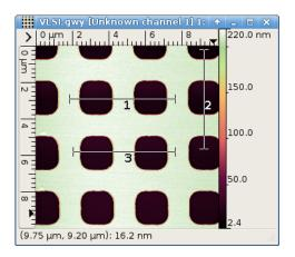
Data window with three selected lines, two horizontal and one vertical.
