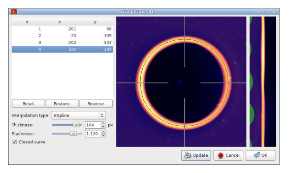
Straighten Path example, showing extraction of data along a closed circular path. The left part of the dialogue contains coordinates of the path-defining points and function options, the middle part shows the selected circular path (with perpendicular markers denoting the thickness), and the right part is a preview of the extracted straightened data.
