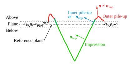
Scheme of different regions of an indentation: above, below, plane, impression, inner pile-up and outer pile-up.
