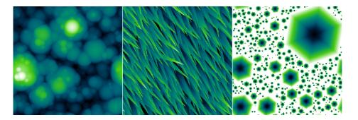
Artificial surfaces generated by object placement: spheres of varied size (left), narrow thatches of varied direction (centre), negative non-overlapping hexagonal pyramids of varying size (right).
