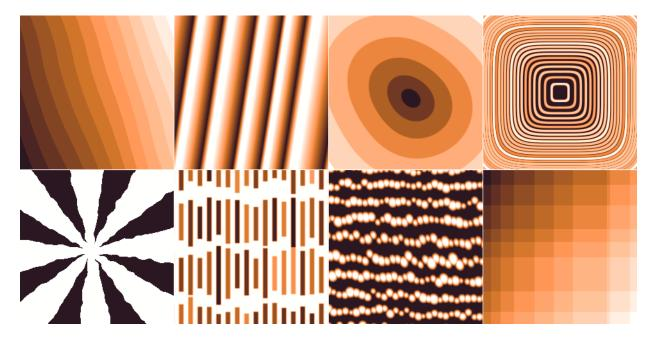
Artificial pattern surfaces. Top row: sharp steps with long-wavelength deformation, scaled grating with large width variance and wide asymmetrical slopes, a slightly deformed amphitheatre with negative parabolicity, and concentric rings with positive parabolicity and varying height. Bottom row: Siemens star with enlarged upper surface, long rectangular holes with varying vertical dimension and position, rows of slightly deformed circular pillars, and double staircase with irregular step width.
