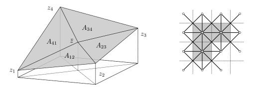
Surface area calculation triangulation scheme (left). Application of the triangulation scheme to a three-pixel masked area (right), e.g. a grain. The small circles represent pixel-centre vertices  $z_i$ , thin dashed lines stand for pixel boundaries while thick lines symbolize the triangulation. The surface area estimate equals to the area covered by the mask (grey) in this scheme.
