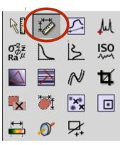
Displays the distance and height difference between two points
