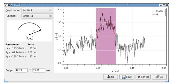
Analysis results: height:  $0.8 \pm 0.2 \text{ nm}$ width:  $32 \pm 4 \text{ nm}$
